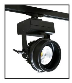
The MCR is suited for medium to long throws. This power saving fixture can produce up to 175 lumens per watt. It features passive cooling, a long-life LED, and 1% dimming. Multiple mounting options, accessories, and dimming types are available.
