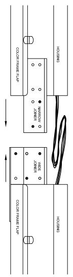
• INDICATES A HOLE TO BE USES AS A DRILL GUIDE IN STEPS 3 AND 4
