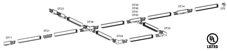
\*There is only one control bus on the track, therefore, all circuits will be sharing the same control signal.
