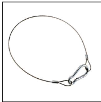
SC Safety Cable 1/8" diameter, 30" long steel safety cable with snap ring. Used as added security when large or heavy fixtures are being used.
