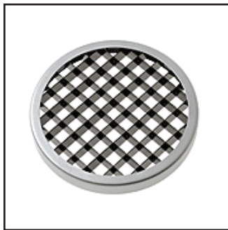
LV Louver Cellular metal louver installed into the accessory compartment of a fixture to reduce excess light spill and glare.
