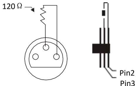
For installations where the DMX cable has to run a long distance or is in an electrically noisy environment, such as in a discotheque, it is recommended to use a DMX terminator. This helps in preventing corruption of the digital control signal by electrical noise. The DMX terminator is simply an XLR plug with a 120 Ω resistor connected between pins 2 and 3, which is then plugged into the output XLR socket of the last fixture in the chain. Please see illustrations below.
