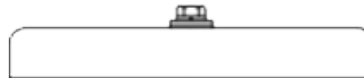
MC Light duty pipe clamp for small fixtures. For pipes up to 1 5/16" O.D.
