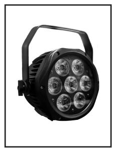
A new addition to our Prism Par family, the Prism Par 7 provides tremendous punch in a small package. This 6-in-1 7x12 Watt LED fixture features a 25° beam angle and a dual yoke/floor stand, multiple unit power linking in rugged die-cast aluminum housing.
