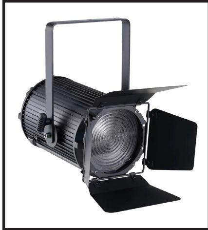
The Lenox is a soft-edged spotlight with more control over beam angle than floods, but less control than profiles. It's electronically zoomable from 12° - 65° degrees with DMX. The Lenox can accommodate barn doors for glare reduction and beam shaping. Selectable and smooth 16-bit dimming curves make it comparable with older, traditional theater fresnels. It is a perfect fit in theaters, studios or other environments that require smooth, even washes of light.
