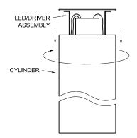
STEP 4: Turning clockwise, *carefully* thread the LED/driver assembly onto the nipple as shown.
