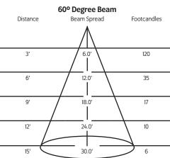
$<sup>\</sup>ast$  Testing done on 3000K unit: Lumen output changes based on color temperature.
