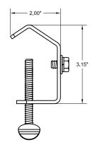
PCL Light duty Clamp for 1/8" to 3/4" pipe (1/8" to 1" OD tube). 20 pound weight rating. Pipe bolt is 1/4"-20 TPI x 1-1/2". Fixture bolt is 1/4"-20 TPI x 1/2".
