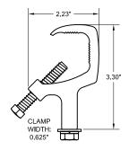
PCE Light duty Clamp for 1/8" to 1-1/2" pipe (1/4" to 2" OD tube). 50 pound weight rating. Pipe bolt is 5/16"-18 TPI x 2-1/2". Fixture bolt is 5/16"-18 TPI x 1/2".
