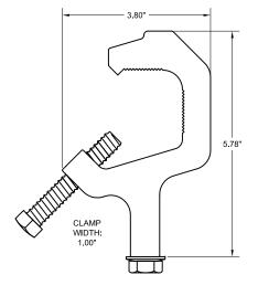
MN Medium duty Clamp for 3/8" to 1-1/2" pipe (3/4" to 2" OD tube). 150 pound weight rating. Pipe bolt is 3/8"-16 TPI x 2-1/2". Fixture bolt is 3/8"-16 TPI x 3/4".
