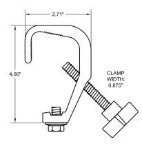
MC Medium duty Clamp for 1/4" to 1" pipe (5/8" to 1-5/16" OD tube). 125 pound weight rating. Pipe bolt is 5/16"-18 TPI x 2". Fixture bolt is 5/16"-18 TPI x 1/2".
