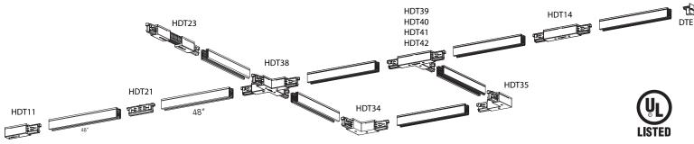
\*There is only one control bus on the track, therefore, all circuits will be sharing the same control signal.
