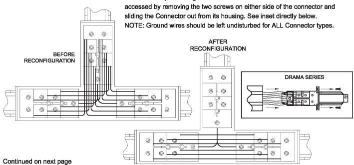
It is imperative that all DMX control wiring on any layout be run in a daisy chain fashion. No loops or branches such as T's or X's are allowed. The layout possibilities are endless, but the diagrams below show the basics of how loops and branch circuits are avoided. See the next page for more requirements on Data Track using DMX control.
