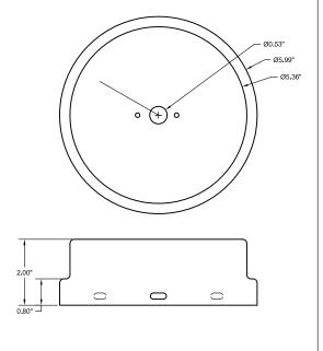
L020 AD1 Monopoint Canopy can be mounted to any standard 3-1/2" or 4", round or octagon electrical box using the provided L020 Adapter Plate using the provided 8-32 screws.
