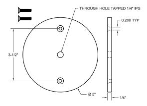
CM3 Canopy can be mounted to any standard electrical box using the provided CM3 Adapter Plate.
