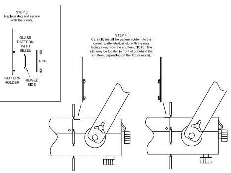
WARNING! IMPROPER GOBO INSTALLATION WILL RESULT IN MISALIGNMENT AND POSSIBLE DAMAGE TO FIXTURE, GOBO, AND/OR PATTERN HOLDER, ALSO, IMPROPER INSTALLATION MAY ALSO RESULT IN GOBO BEING STUCK INSIDE FIXTURE!
